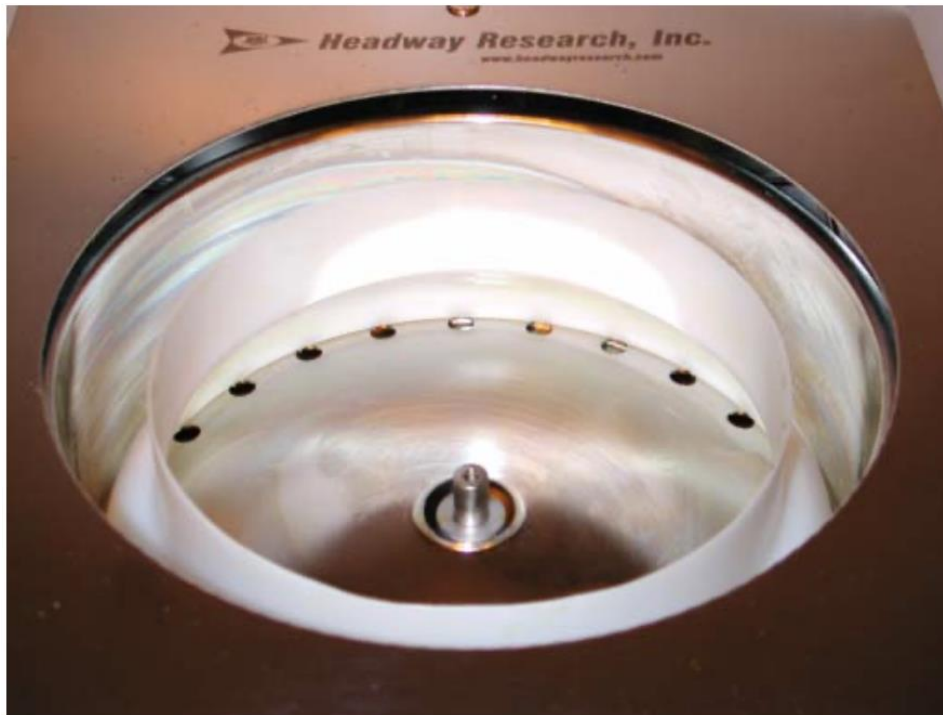
Figure 1: Spinner assembly without chuck.
